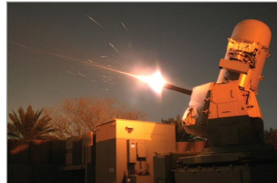
The Land-based Phalanx Weapons System (LPWS) intercepts incoming threats during Counter-Rocket Artillery Mortar (C-RAM) System-of-Systems Demonstrations at Yuma Proving Ground.
