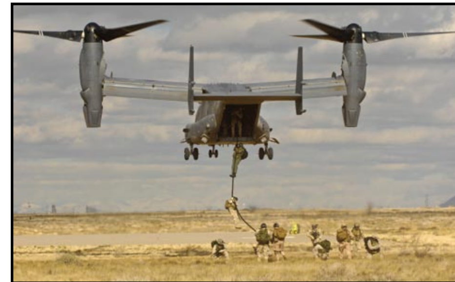
Special Operations Forces operators participate in a test to determine the suitability, effectiveness, and safety of the Improved Weighted Fast Rope System during fast rope insertion operations from the CV-22 (Osprey) aircraft.
