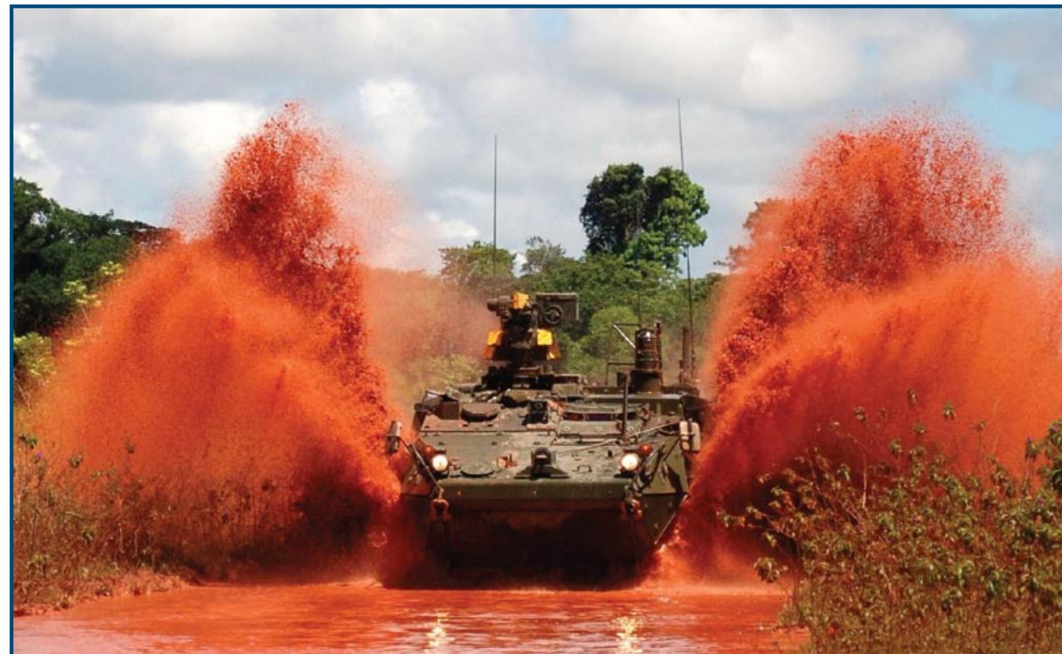
Stryker vehicle fording flooded roadway while undergoing a 2,000 mile endurance cycle.
