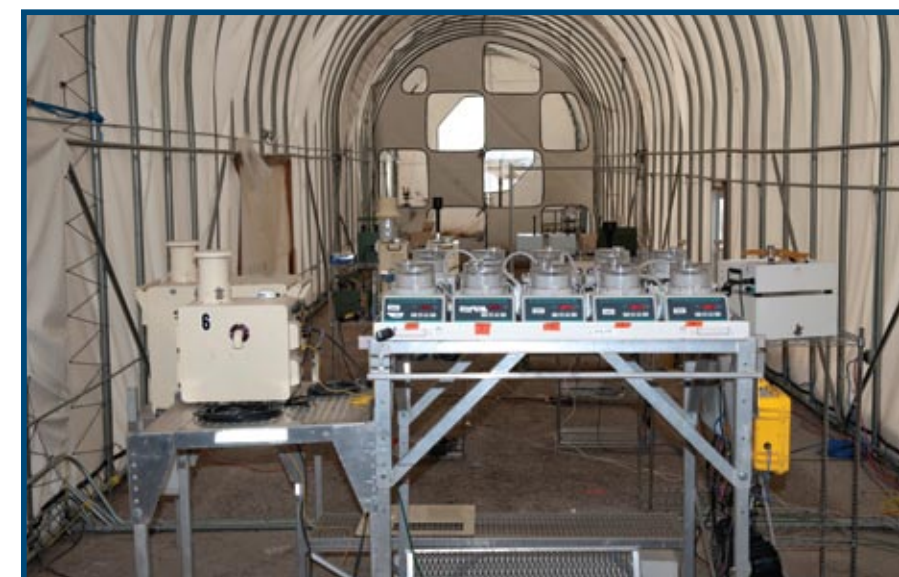
Tunnel Test of Joint Biological Tactical Detection System (JBTDs) in the Ambient Breeze Tunnel of Life Sciences Division, West Desert Test Center, U.S. Army Dugway Proving Ground, Utah.
