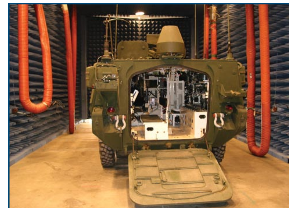
The Electronic Proving Ground conducts test during the development of systems such as Stryker Commander's Vehicle in Chamber 4, being prepared to perform emissions testing.
