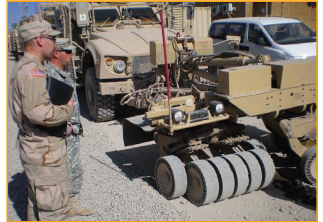
Operational testers look over the rollers on a mine clearance system.
