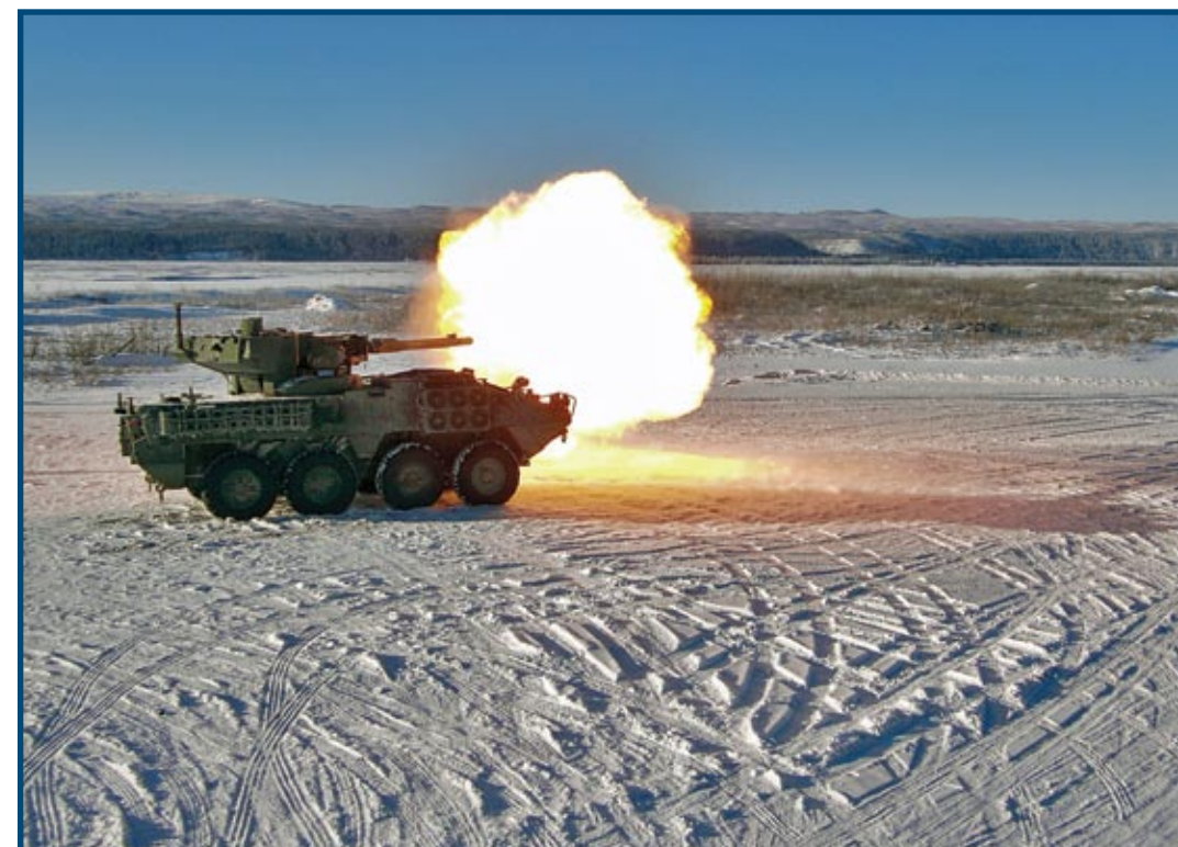
The Stryker Mobile Gun System fires a 105 mm round downrange in sub-zero temperatures during a rate of fire test.
