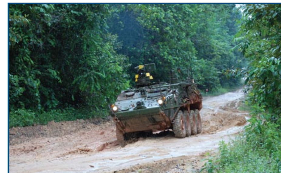
Tropical on-the-move testing of a Stryker with onboard data acquisition instrumentation in a mission based scenario.
