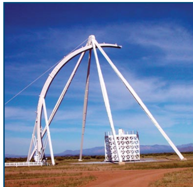
The Arc Range at the Antenna Test Facility measures electromagnetic fields that radiate from antenna systems that populate a variety of land and air vehicles. With its 75 feet radius and 80 ton positioner system the range is capable of making these measurements on any vehicle in the Department of Defense inventory.
