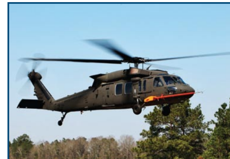
UH-60 upward turned exhaust testing to reduce the heat signature of the aircraft.
