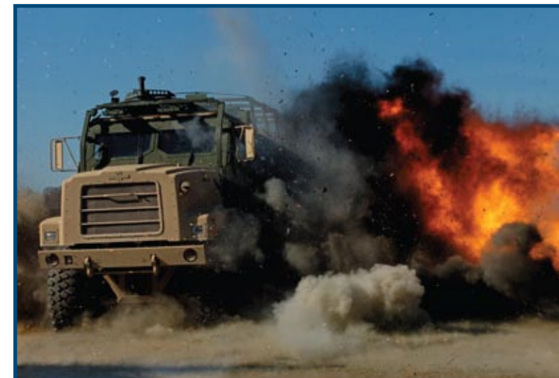
The US Army Aberdeen Test Center is the Army's Center for Excellence for congressionally mandated live fire vulnerability lethality testing, as shown in this live fire shot on a Medium Tactical Vehicle Replacement (MTVR).
