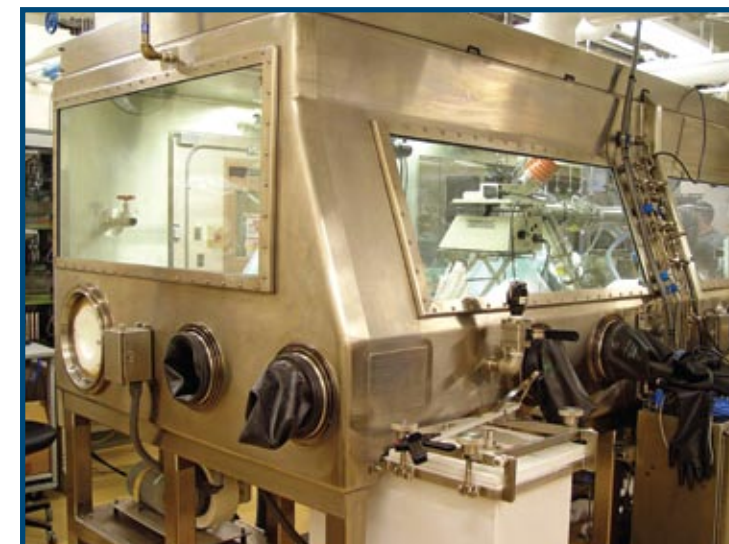
Containment Aerosol Chamber at Life Sciences Division, West Desert Test Center, U.S. Army Dugway Proving Ground, Utah. In this chamber, actual or simulated Biosafety Level-3 agents are released as a fine aerosol, to test biological detectors.
