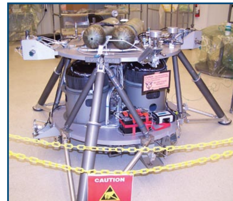
NASA Robotic Lunar Lander undergoes a series of integrated system testing at the Propulsion Test Facility.
